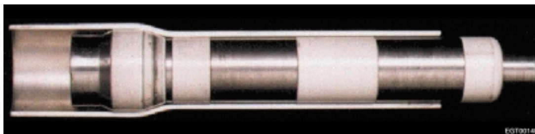
Fig. 1 – Early expansion mandrel used to expand Solid Expandable Tubulars (SETs)
