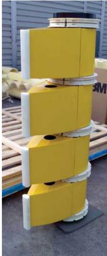
Figure 2: Example of weathervaning fairings [3]
