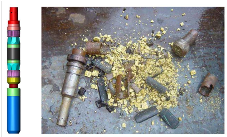
Figure 2. Frangible bridge plug (left) and leftovers after desintegration (right).
