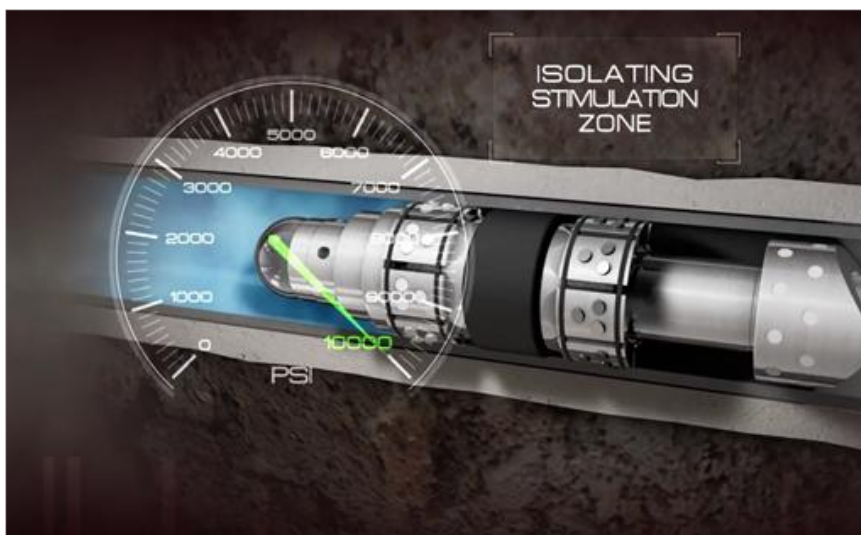
Figure 9. Ball pumped down and stimulation performed.
