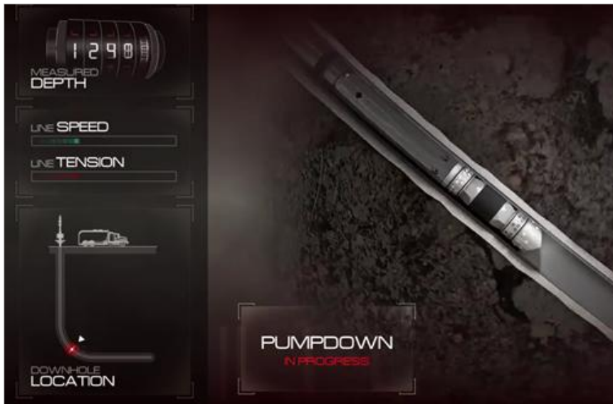
Figure 7. Pumping down the DFP.
