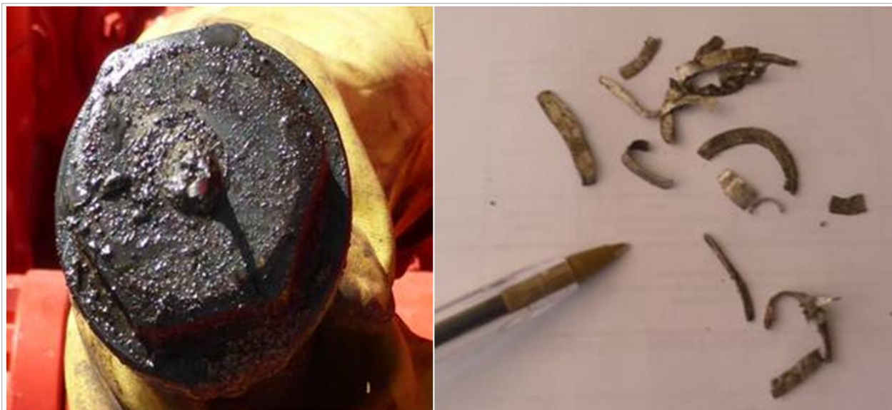
Figure 26. Pieces of metal plugging the choke.
