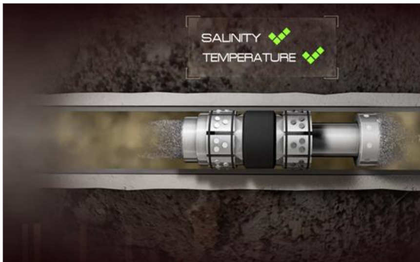
Figure 11. Well is allowed to flow back. Temperature and salinity increase accelerate the dissolution process of the frac ball and DFP.
