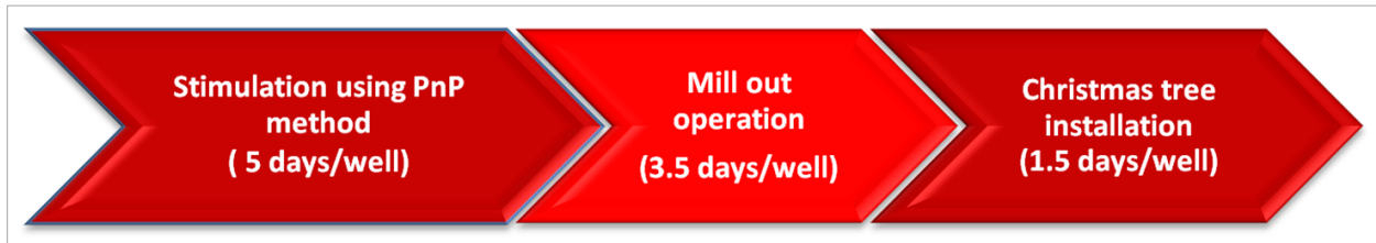
Figure 1. Current estimation of PnP operations duration in Vaca Muerta wells.
