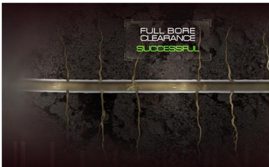
Figure 12. Full wellbore clearance is achieved after total DFP dissolution.
