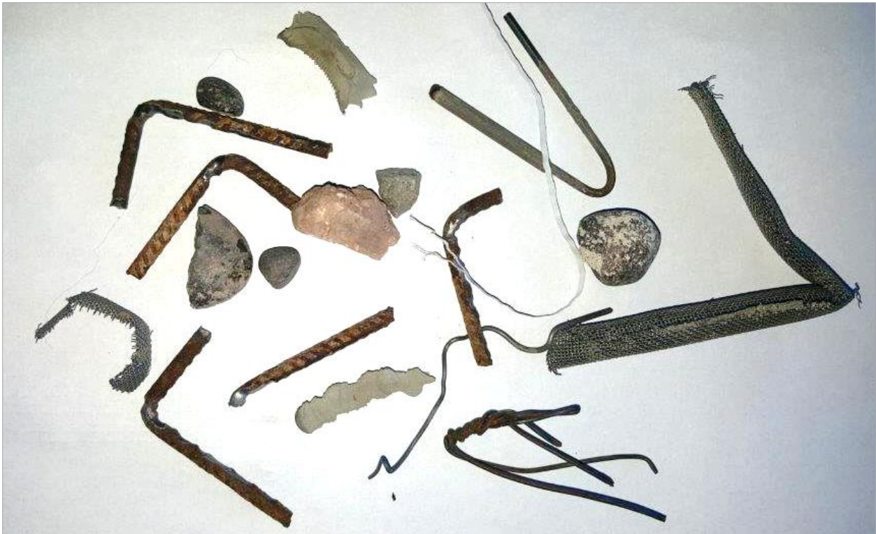
Figure 27. Example of debris collected from sand used for stimulation operations.
