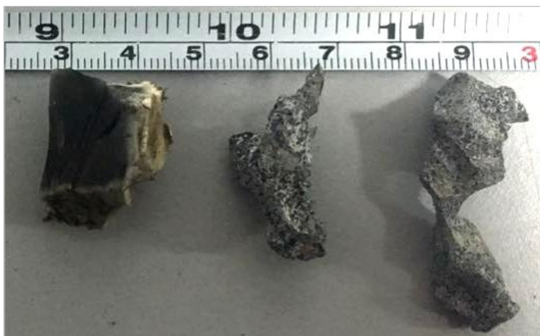
Figure 22. Pieces of a DFP recovered after flowback during stimulation of Stage 7.
