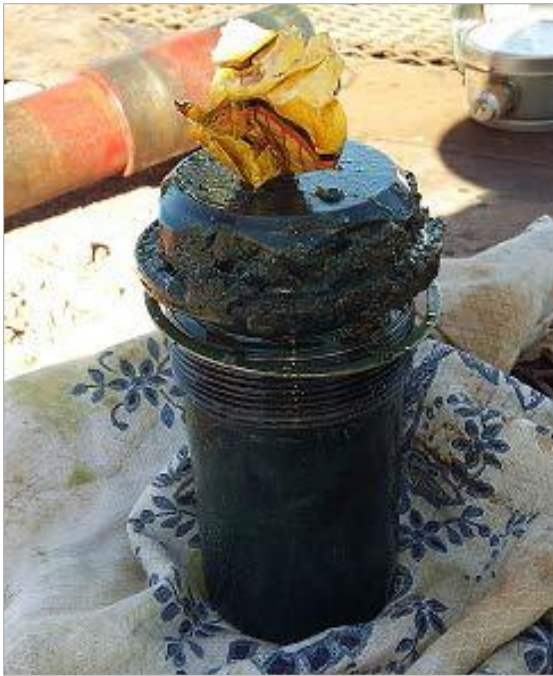
Figure 29. Example of a sticker from a perforating gun found plugging the choking orifice at surface.
