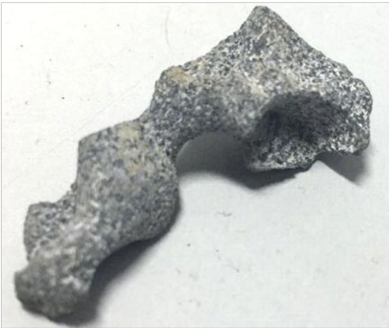
Figure 24. Piece of DFP recovered after flowback during stimulation of Stage 7.
