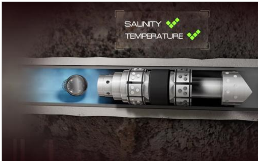
Figure 10. Well is allowed to flow back. Temperature and salinity begin the dissolution process of ball and DFP.
