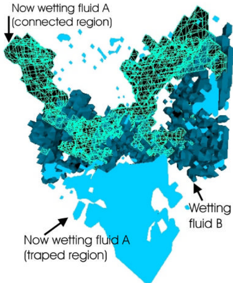
Figure 9: 3D visualization of wetting fluid invasion in to sample sandstone
