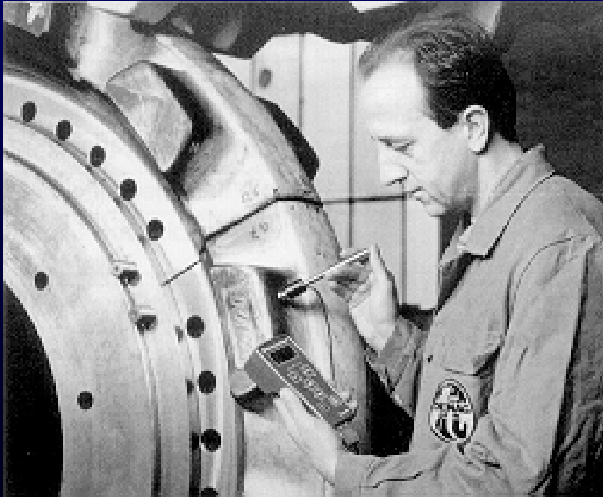
Hardness testing with a rebound tester on the drive wheel of a large hydraulic digger.
