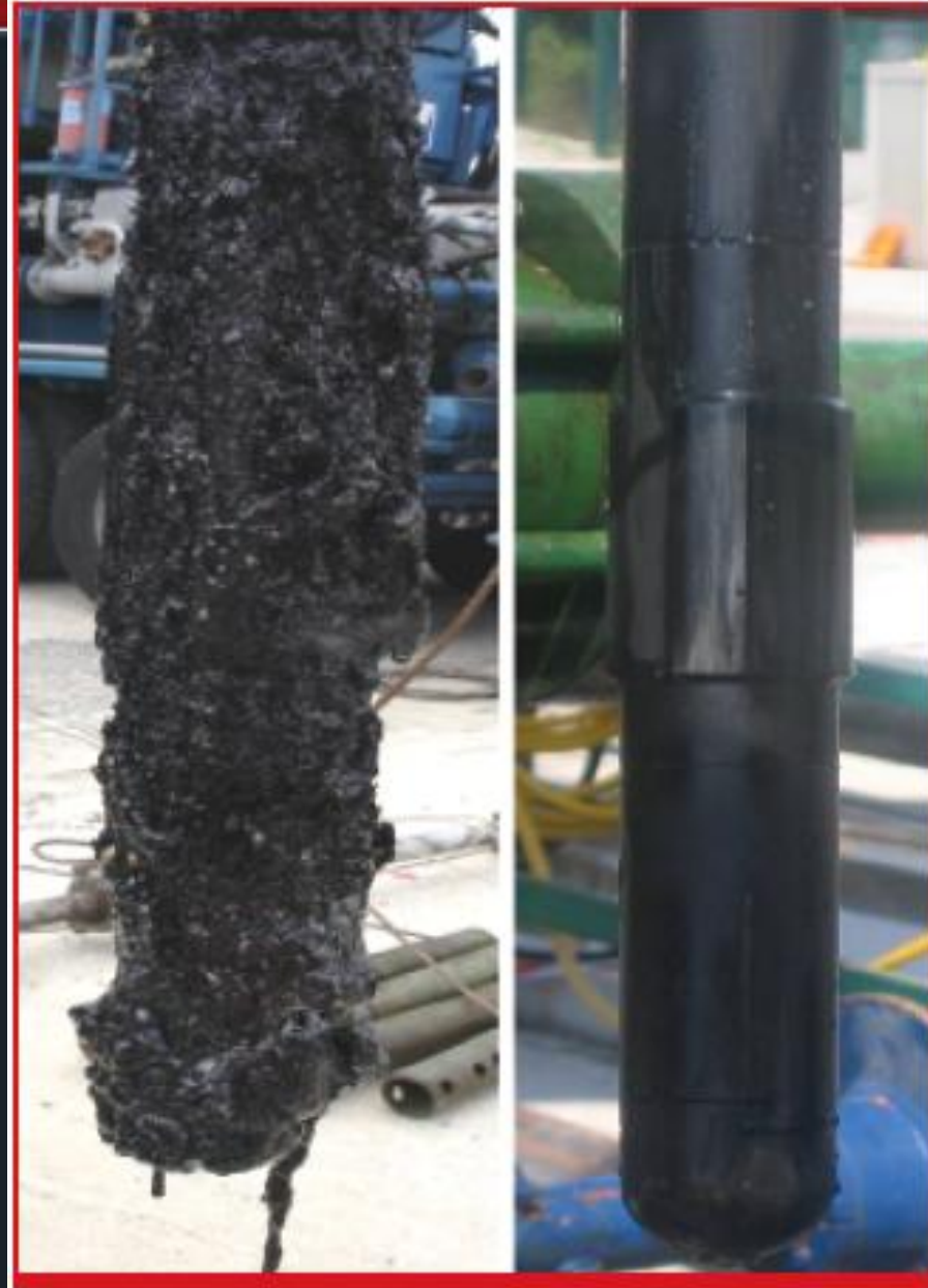
Figure 1 - Bottomhole assembly fouled with asphaltene (left) prior to DuraKleen service and (right) following the service.
