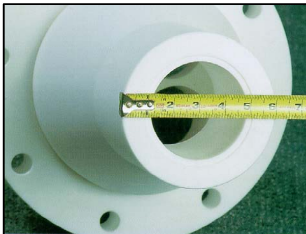
Figure 3. Typical Reverse Jet Nozzle for SRU Tail Gas Treatment Applications
