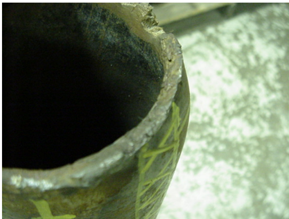
Figure 3 – 45 degree fracture surface of joint C2
