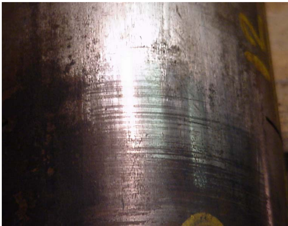
Figure 5 – Formation cuts and polished outer surface on the tube body of joint C1
