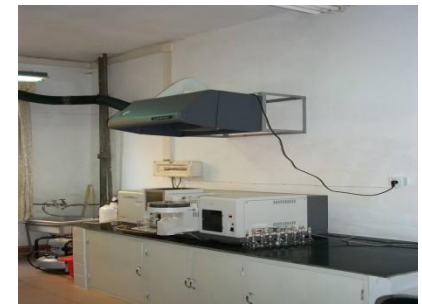
HITACHI Z-5000 atomic absorption spectroscopy equipment
