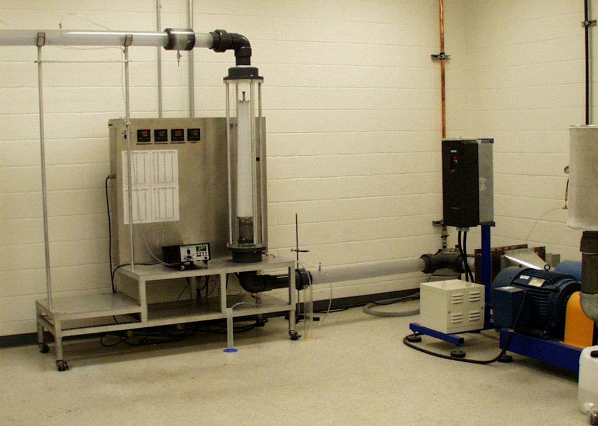
Large Flow Liquid/Gas Separator Test Stand
