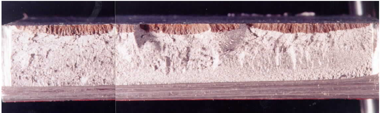
Figure 2. Optical photograph of pipe sample following breaking in liquid nitrogen, showing interlinked stress corrosion cracks.
