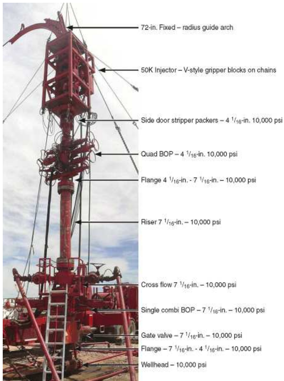
Fig. 2—Wellhead with HPAP technique.
