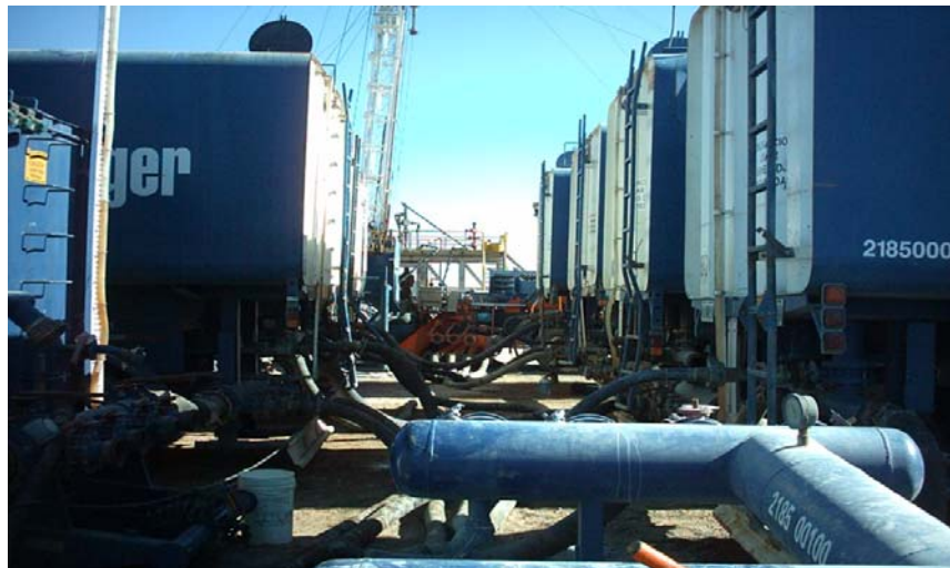
Figures 5: Rig-up showing the largest EMFS completion to date in Argentina, in terms of total amount of proppant pumped with a total of 500,000 lb placed in the formation.
