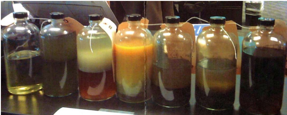
Figure 1 – Several different batches of shale crude received on the same day. Variability in crude charge causes corrosion challenges in the overhead.
