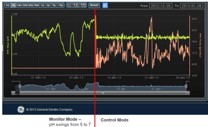
Figure 10 - pH variability can be eliminated via automatic neutralizer pump control.
