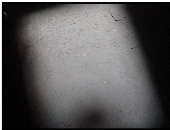
Figure 7 - The photo shows a layer of FeS dust covering the top of the first catalyst bed in a kerosene/diesel hydrotreater which shuts down every 3 to 12 months due to pressure drop built-up. The refinery runs high acid crude so corrosion produces soluble Fe in the kerosene
