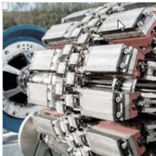
Picture 1. Dual sensor ring of MFL-A Ultra ILI tool
