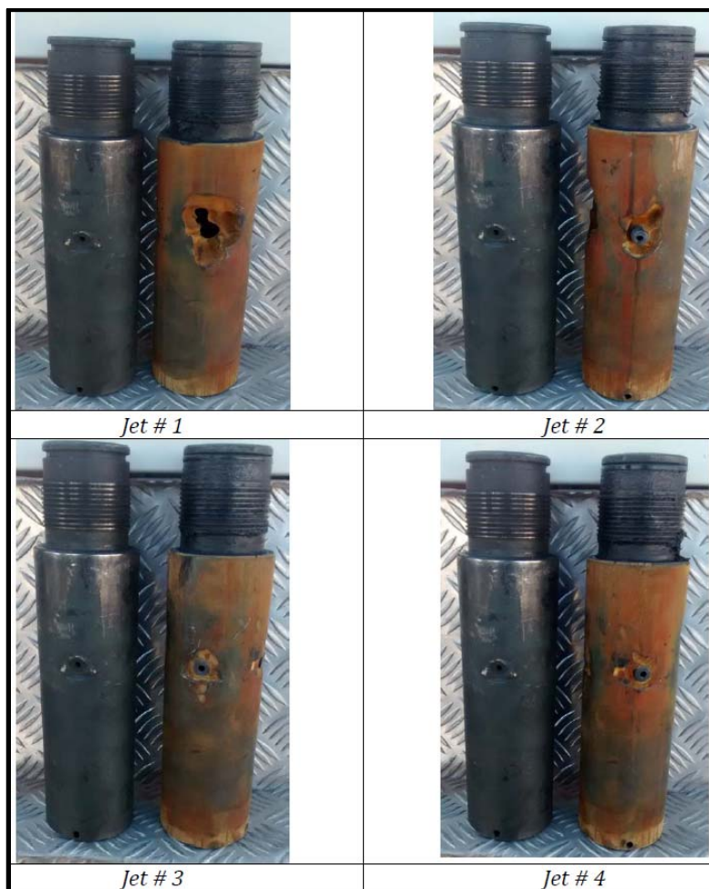
Figure 5 - Jet Erosion (Actual Vs New)
