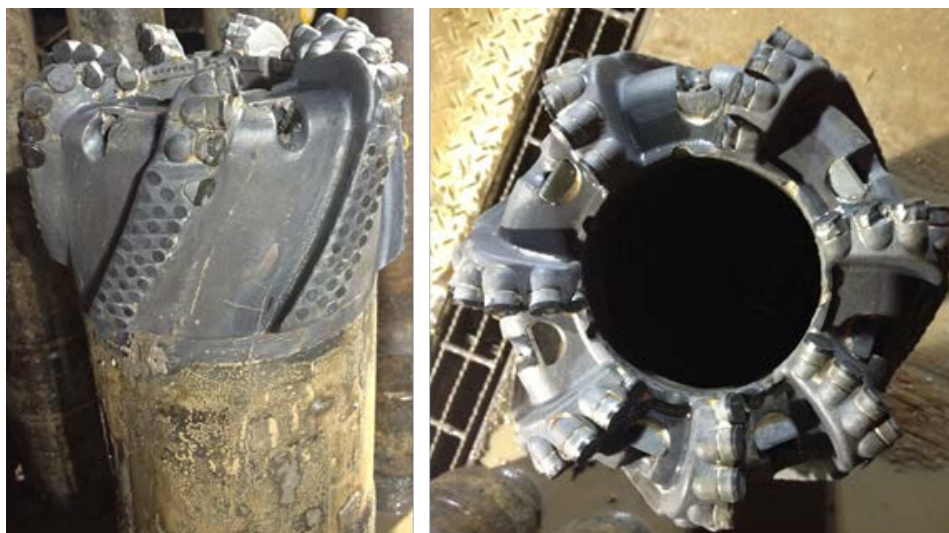
Fig. 5—Standard core head used in shales and interbedded formations.
