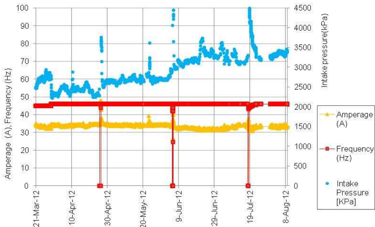
Fig. 19—Well behavior and ESP operating parameters after optimization, well 40.
