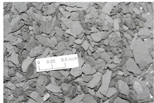
Fig. 4 – Thin and sharp cuttings collected from a Marcellus well. Cuttings from Eagle Ford wells are often like coffee-grinds
