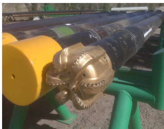
Fig#4 Trepano perforable EZC-406
