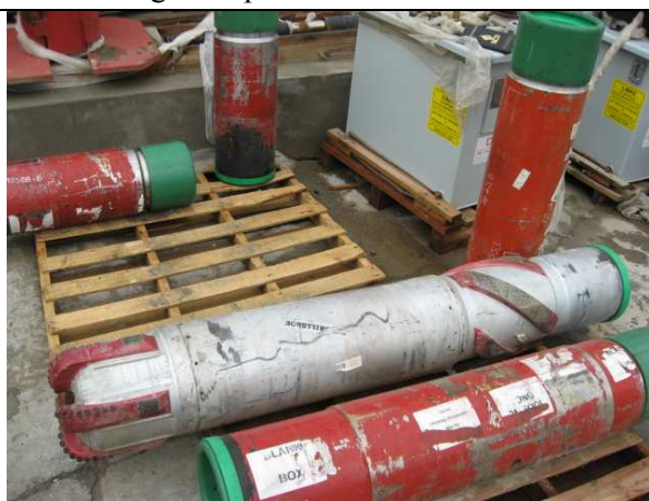
Fig#5 Trepano Weatherford DPC-516
