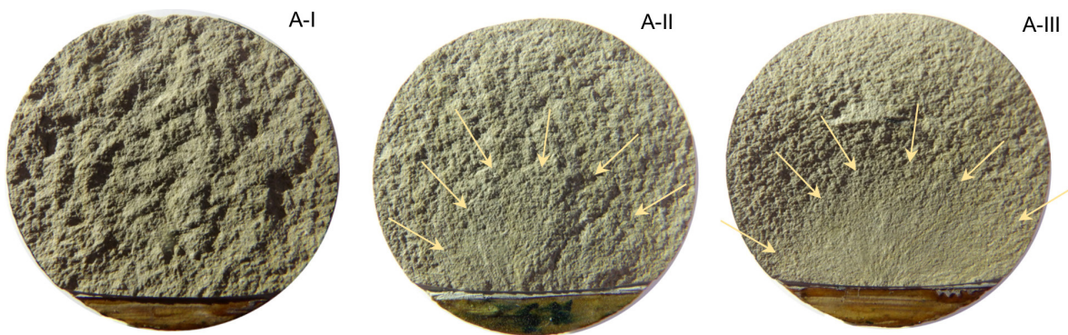
Figure 5. Evolution of fracture surface against confinement pressure. The notation I, II and III correspond to atmospheric condition, 20-30 and 50 MPa respectively. The arrows indicate approximate position of mirror zone.
