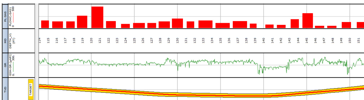
Figure 2a. Lateral production drainhole in an unconventional shale gas reservoir. Track 1 is the well trajectory in TVD (red curve); yellow shading is the target window. Track 2 is the GR, the only petrophysical data acquired. Track 3 is measured depth in feet. Track 4 is gas production per stage in BOEPD.
