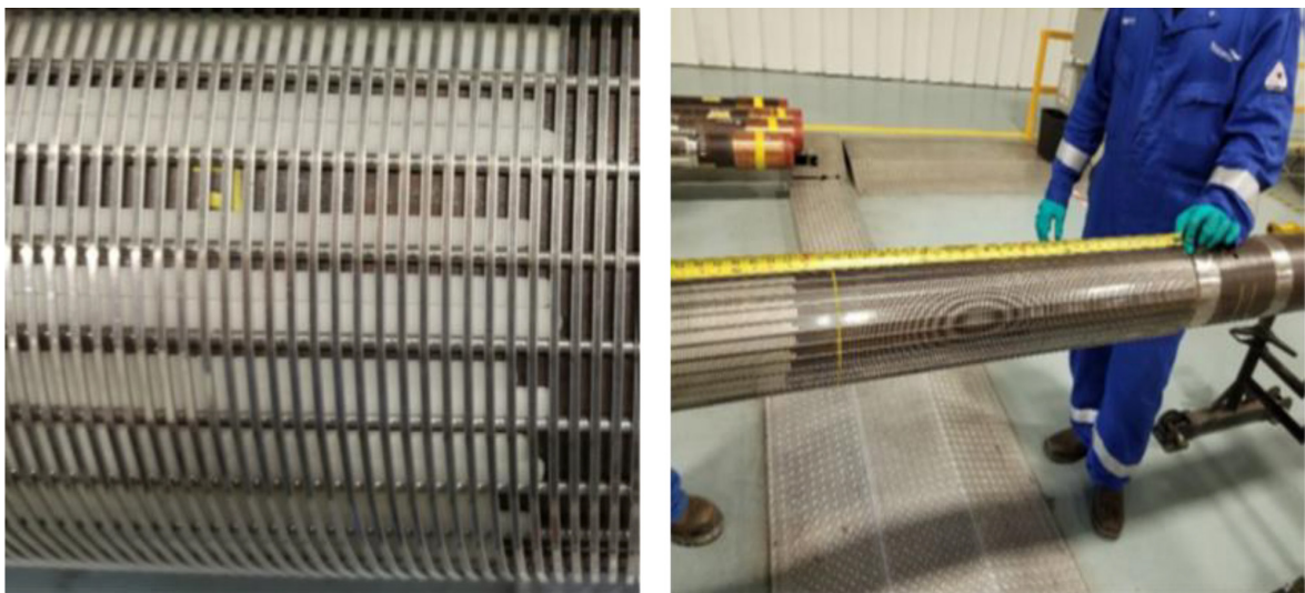
Figure 25. Tracers' strips into screen drainage layer.
