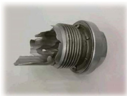
Figure 4. Choke bean (eroded)
