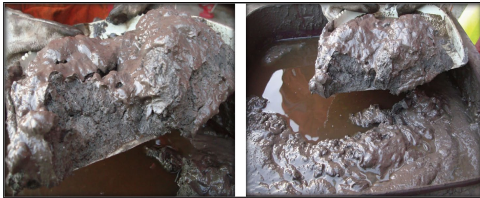
Figure 6. Mud with high concentration of micronized solids
