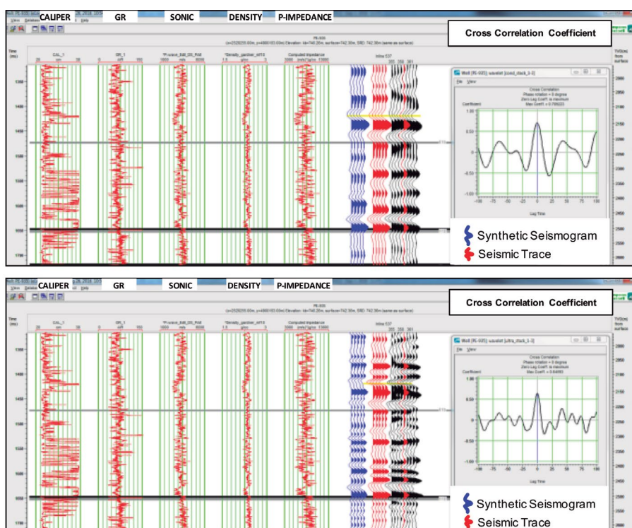
Figure 4. Well to seismic tie at P-935 well. The correlation between the extracted trace (red) and the synthetic seismogram (blue) shows a good fit and consistency with both conditioned (upper image) and frequency-enhanced data (lower image).
