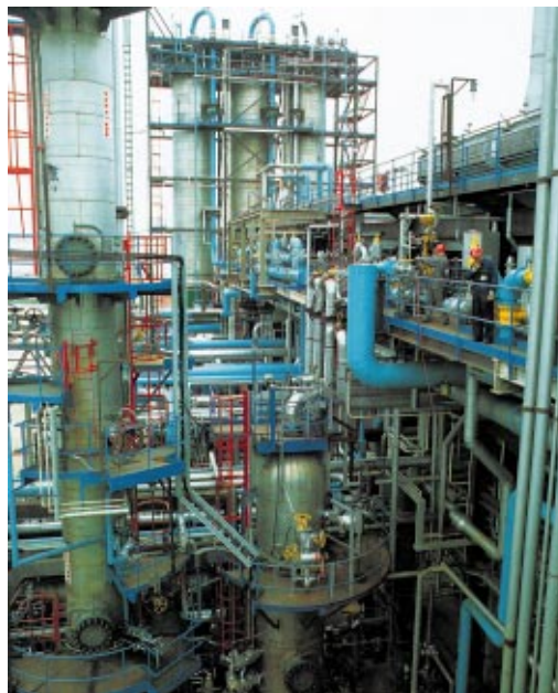
Hydroprocessing removes sulphur and increases yields of road fuels, but consumes hydrogen and increases global CO 2 emissions.
