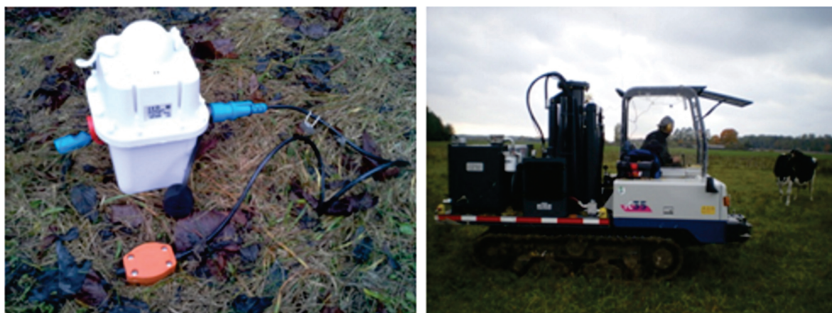
Figure 3. Equipment utilized for 3D survey. Left) Wireless seismic recorders. Right) AWD.
