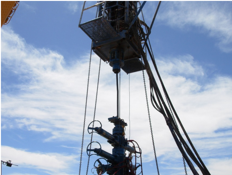
Fig. 9 Double BOP (double safety barriers) and Extra Clamp
