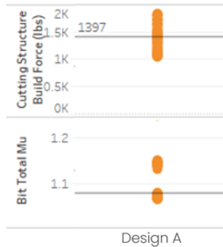
Figure 18. Simulations results on steerable response from the PDC drill bit, Design A.
