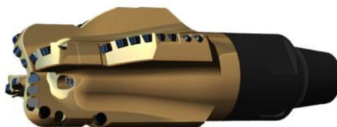
Figure 8. Three Dimensional Render of the selected hole enlargement PDC drill bit.
