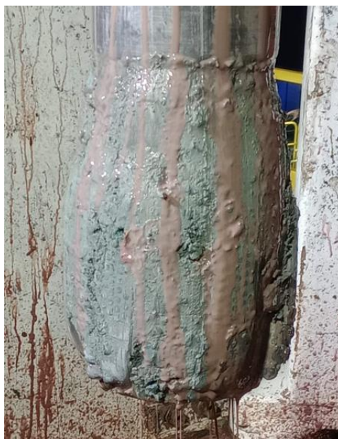
Figure 1. balled up tool due to clays.
