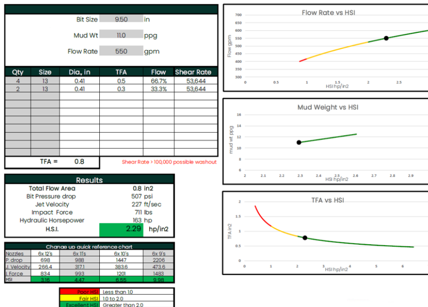
Figure 12. Hydraulic performance at the hole enlargement PDC drill bit.
