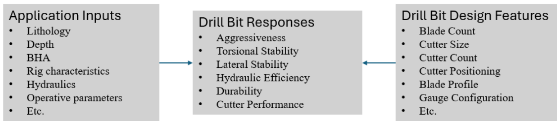
Figure 5. Relationship between application inputs and drill bit features defines drill bit response
