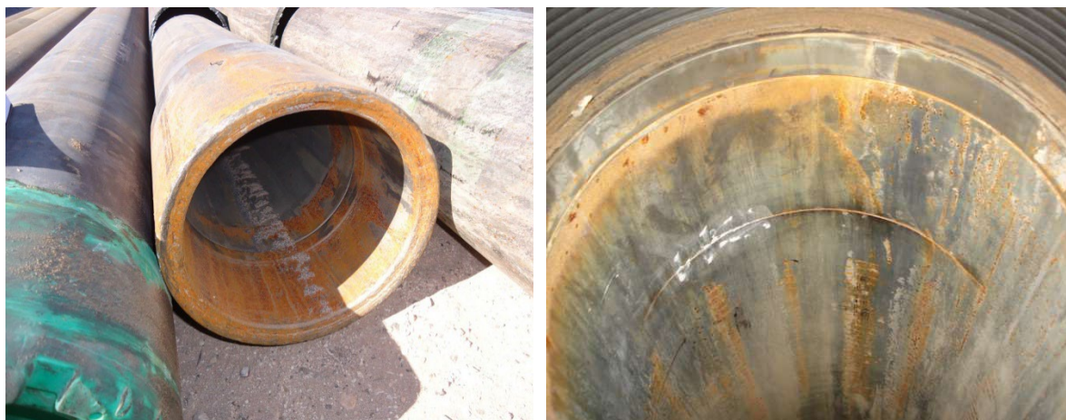
Figura 3: Failure of 9 5/8" TXP BTC during casing drilling operations – Well Laj-75 – Tight gas development 2015 (Codega Dario, 2015).
