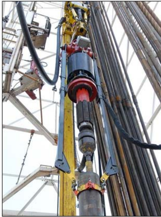
Figure 7 Next Generation Top Drive Casing Makeup System, Internally Gripping
