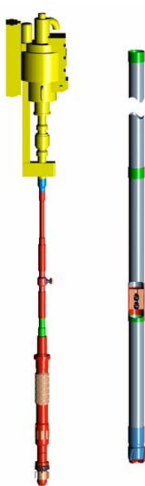
Figure 3 Drilling With Casing System
