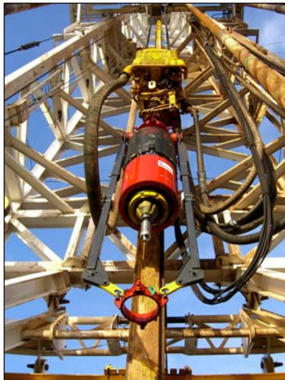
Figure 6 Next Generation Top Drive Casing Makeup System, Externally Gripping
