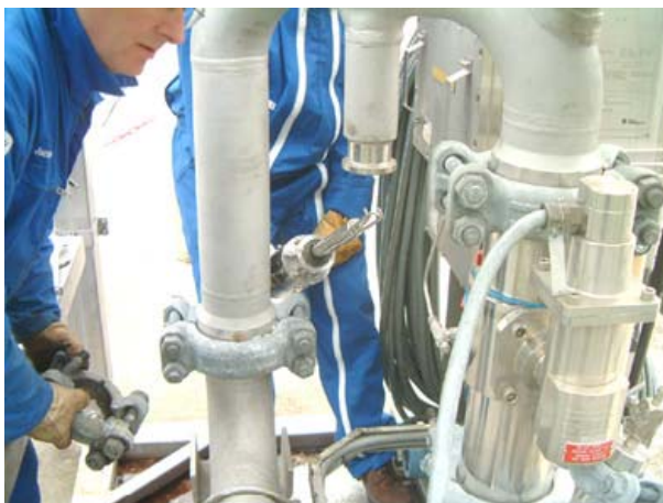
Figure 5: ASD connected to the PhaseTester liquid sampling port
