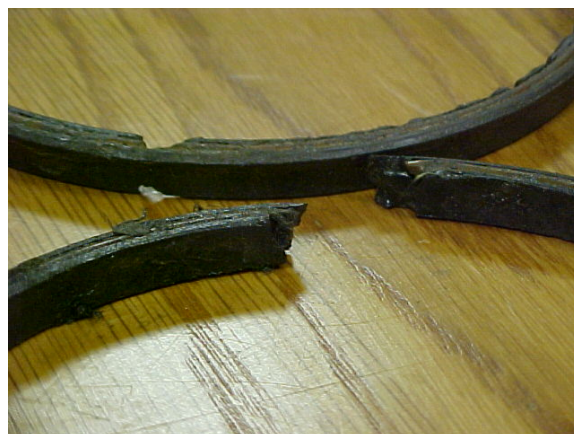
Figure 7. Close-up of Damaged Seals
