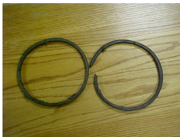
Figure 6. Damaged/Split Choke Line Seals
