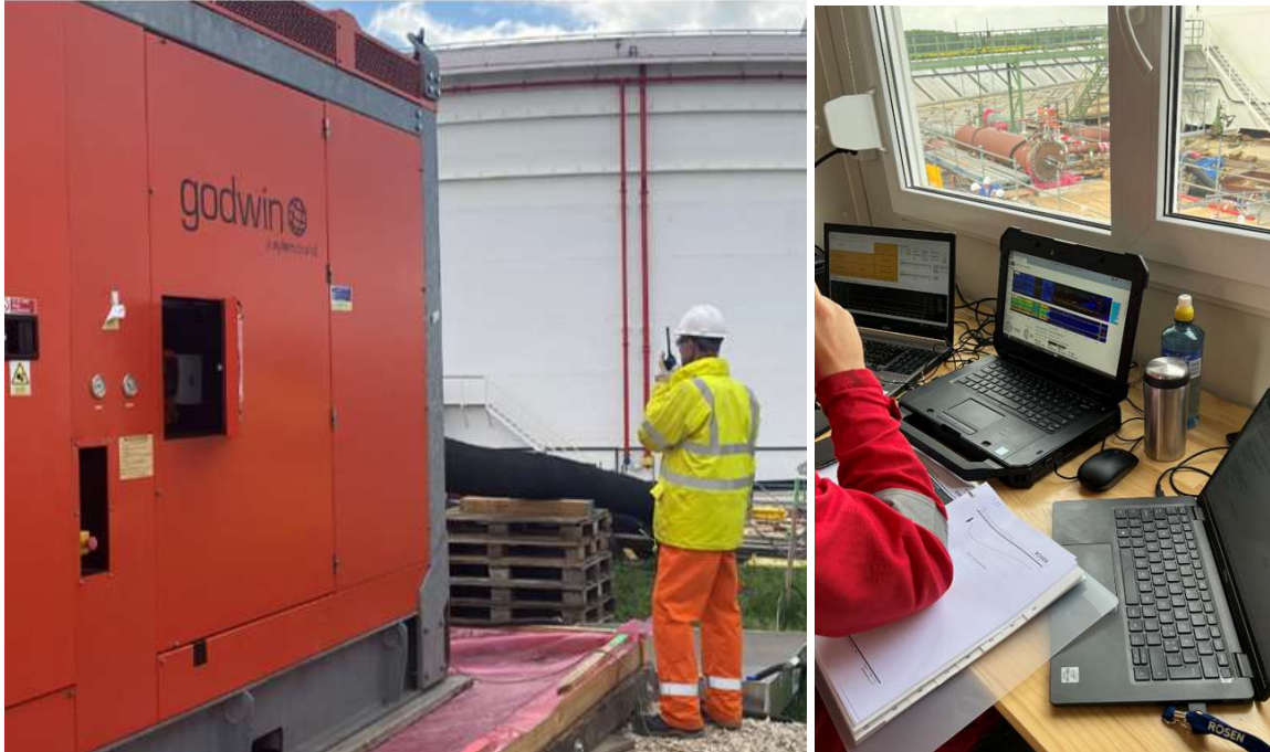
Figure 16: ROSEN Field Engineers operating the pump for RCP runs (left) and ROSEN Inspector monitoring inspection progress of tethered UTWM inspection (right)
