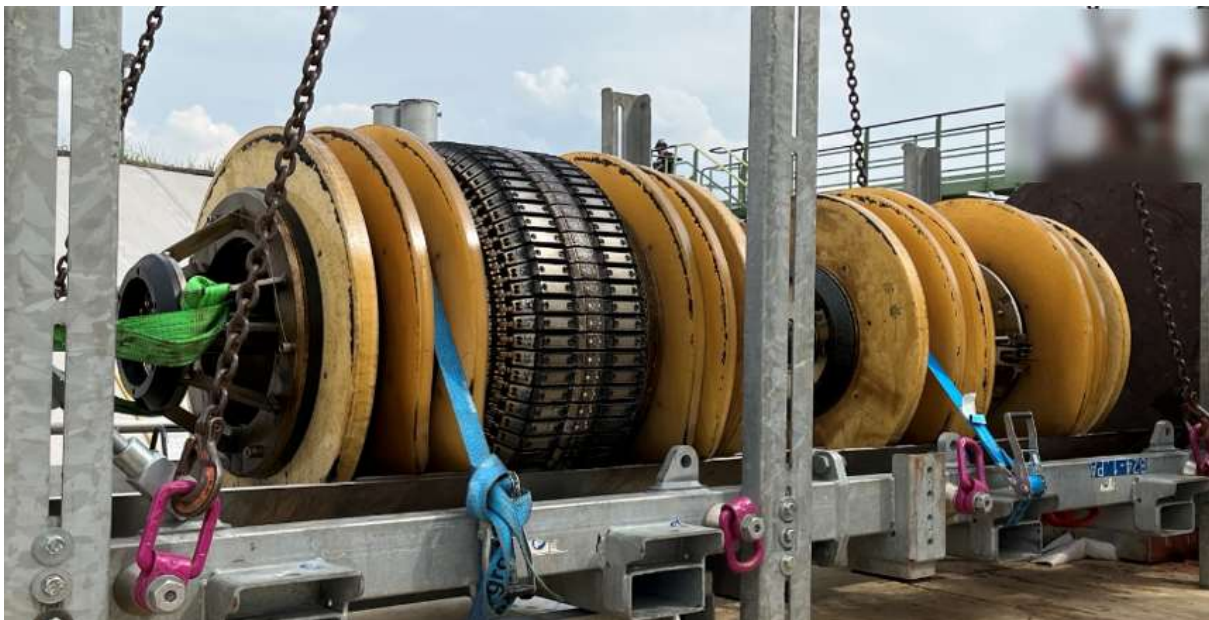
Figure 15: Picture Tandem 36" MFL-A tool after the run
