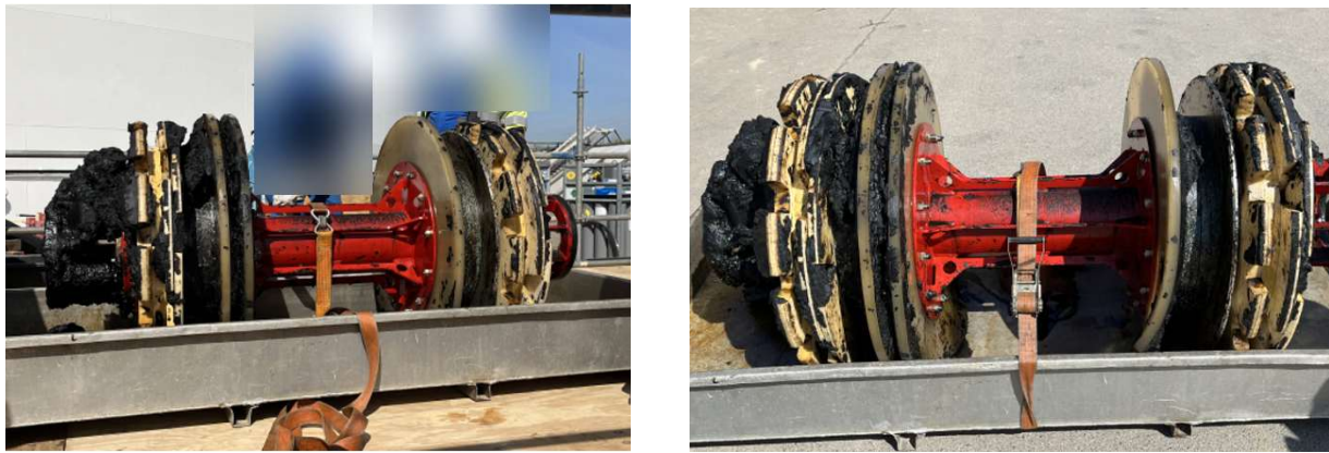
Figure 15: Picture Tandem 36" MFL-A tool after the run
